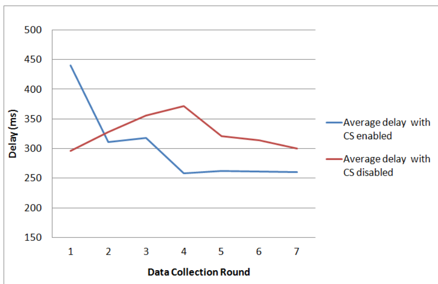
Figure 13: Average collection delays at the sink over several collection rounds with enabled and disabled caching strategy using 10 TelosB nodes.
