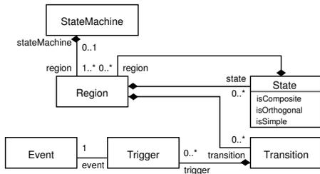
Fig. 1. Subset of the UML StateMachine Metamodel
