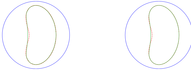
Figure 2. Exact (red) and reconstructed (green) geometries after 10 iterations (left) and 15 iterations (right). \lambda = 0.01 and the Cauchy data to f_1 = \sin t , f_2 = \cos t and f_3 = 1 . No added random noise.
