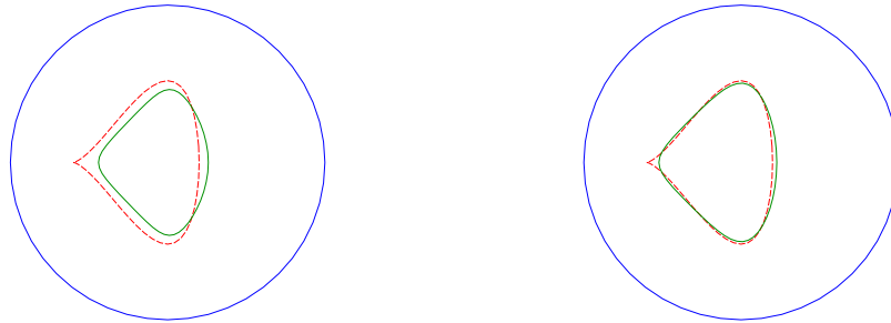
Figure 1. Exact (red) and reconstructed (green) geometries after 2 iterations (left) and 6 iterations (right). \lambda = 0.01 and the Cauchy data to f_1 = \sin t , f_2 = \cos t and f_3 = 1 . No added random noise.
