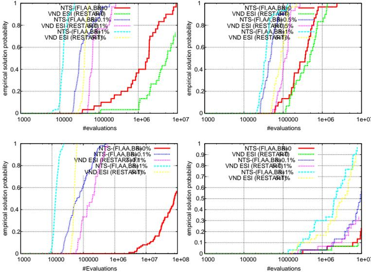
**Figure 2: RTDs for NTS vs VND with random restart. The x-axis gives the logarithm of the number of fitness evaluations, the y-axis the cumulative empirical solution quality probability.  $\delta$  denotes the gap (in percentage) between the required solution quality and the optimal solution. Top-Left figure (resp. Top-Right, Bottom-Left and Bottom-Right) shows the results for instance 19 (resp. 38, 42, and 86).**
