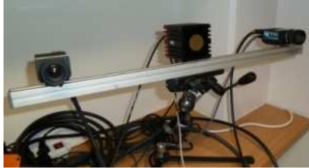
(a) A ToF-stereo setup
