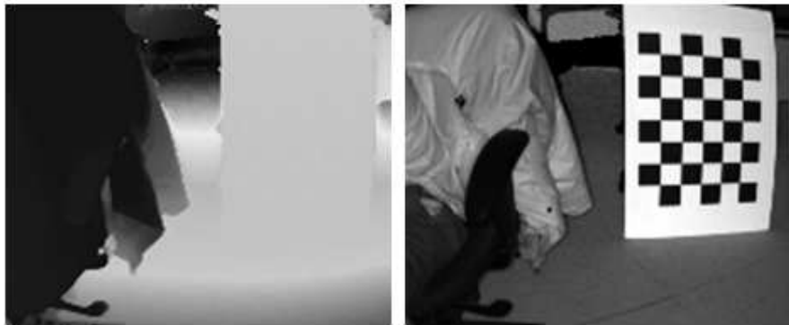
(b) IR Amplitude Error: 3D points of the same depth (chessboard on the left) show different IR amplitudes (chessboard on the right) according to the color of the target object.
