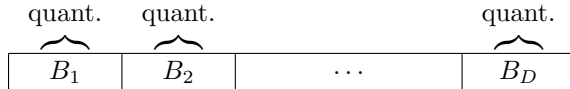
Figure 2: Illustration of the PQ procedure on one vector. The vector is considered as a product of D subvectors of equal length, and each subvector is quantized separately using a k -means algorithm on the database \mathcal{X} .
