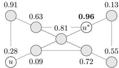
Fig. 1. In this example  $M = 1$ . The label near a node  $v$  represents  $x_1^{(v)}(0)$ , and  $u^*$  is the node with maximal initial condition. Considering agent  $u$ , its estimated eccentricity  $\widehat{e}^{(u)}(t)$  will converge to 3, i.e., its distance from  $u^*$ .
