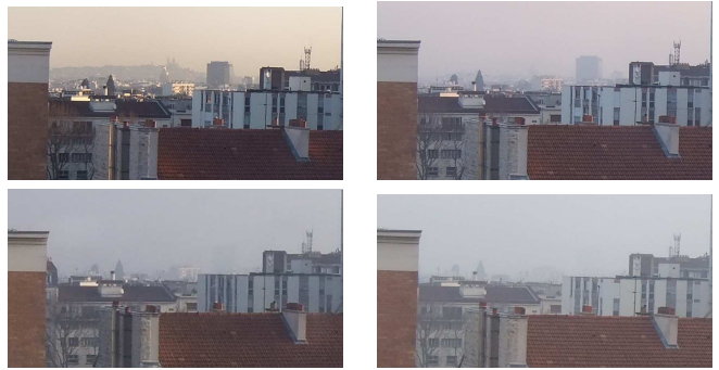
Fig. 1. Contrast fading on the same scene due to various values of the extinction coefficient k .
