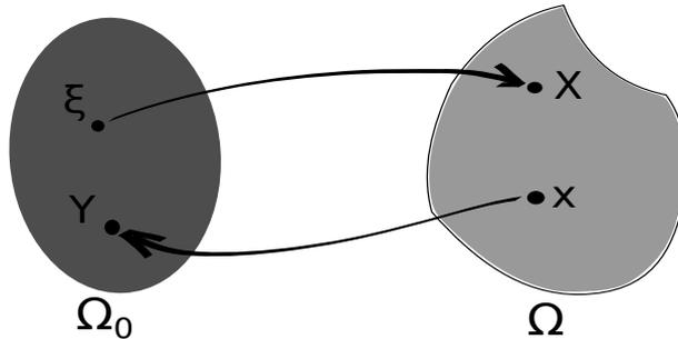
Figure 1: Lagrangian description of transport: the reference configuration is  $\Omega_0$ , points  $\xi \in \Omega_0$  are transported by the direct mapping in  $X(\xi, t)$ . Given the actual configuration  $\Omega$ , a point  $x \in \Omega$  is sent back to its counterimage in the reference configuration by backward characteristics, i.e., the inverse mapping  $Y(x, t)$ .
