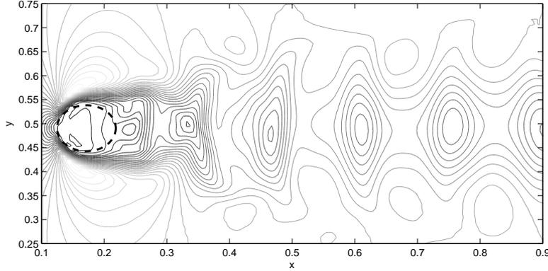
Figure 14: Barycentric density for the kinetic energy of the flow around a circular cylinder: isocontours, 30 lines between the maximum and the minimum
