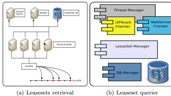
Figure 2(a) presents the approach used to collect *leasesets*. Each floodfill is running in one PlanetLab node, and logs every received request to a PostgreSQL server, located in our high security lab.
