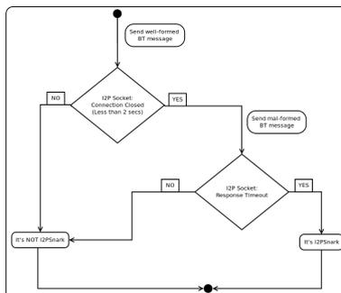
Figure 3: Algorithm for testing an I2PSnark client
