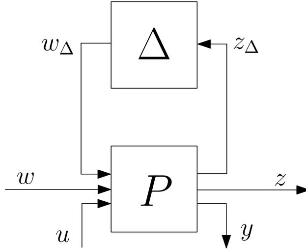
Figure 10: System under LFT form
