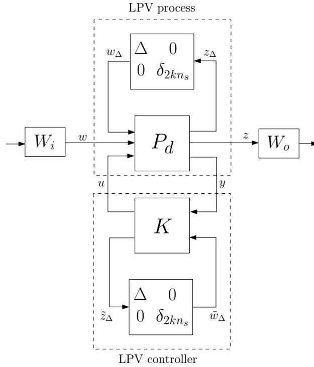
Figure 11: LFR control structure
