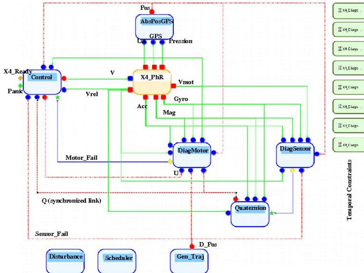
Figure 2: X4 drone control and diagnosis block-diagram.
