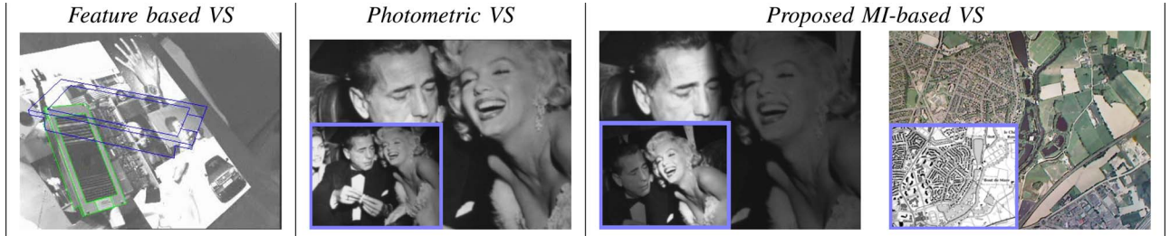
Fig. 1. From feature-based tracking to direct approaches. A visual-servoing task was usually based on measures extracted from the image such as points and contours. It is now possible to run a visual-servoing task with no feature extraction or image processing through direct approaches. Our new approach is now capable of servoing the robot using images acquired using different modalities.
