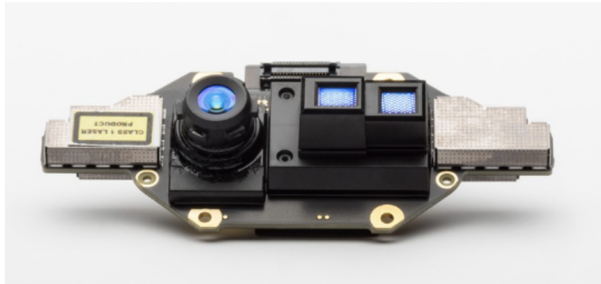
Figure 1.6: Depth Sensor: The Azure Kinect DK depth camera. Image taken from Microsoft [Mic23].
