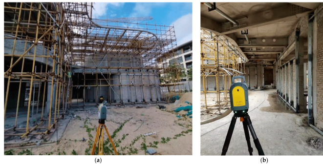
Figure 1.3: Laser scanning. A laser scanner is used to scan point clouds from a construction field. Image taken from [WYLU22].
