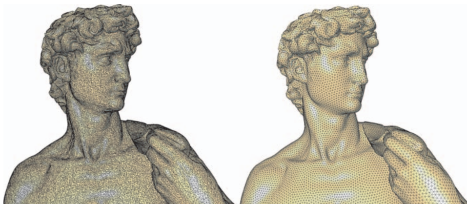
Figure 2.23: Uniform remeshing of the Digital Michelangelo David model. Left: the mesh extracted by marching cubes contains many badly-shaped triangles. Right: the mesh becomes isotropic (well-shaped) after remeshing. Image taken from [AUGA08].
