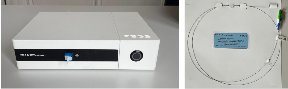
Fig. 4.2 Components of FBGS measurement system: the interrogator (left) and the optical fiber (right).
