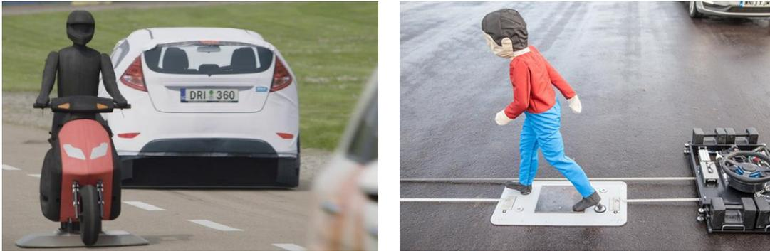
Figure 40 – These pictures display some examples of actuated dummies and soft targets that are used to test **ADS** and **ADAS**. These images are from [www.abdynamics.com](http://www.abdynamics.com) [A23].
