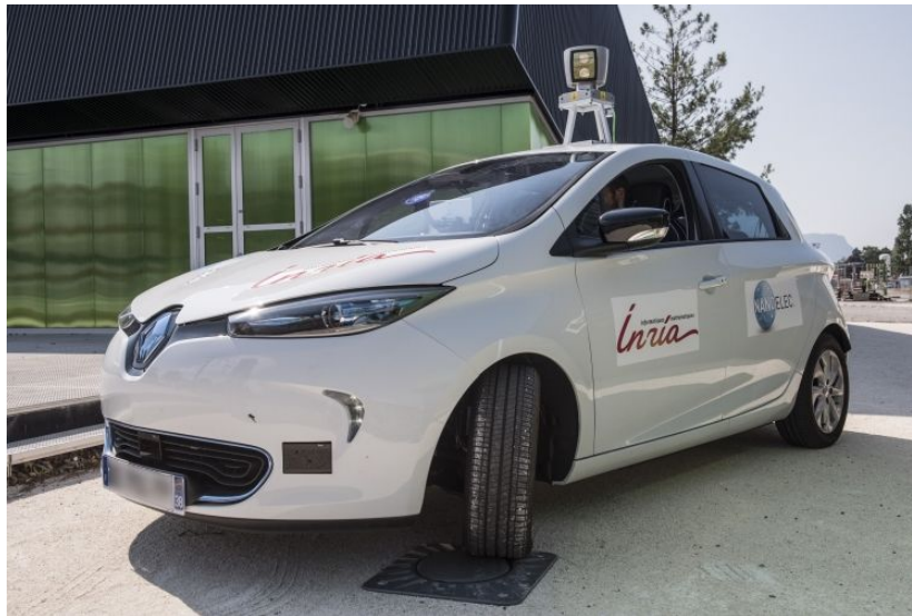
Figure 52 – The automated car prototype that has been used to experiment and demonstrate the software contributions of this thesis in the domain of ADS .
