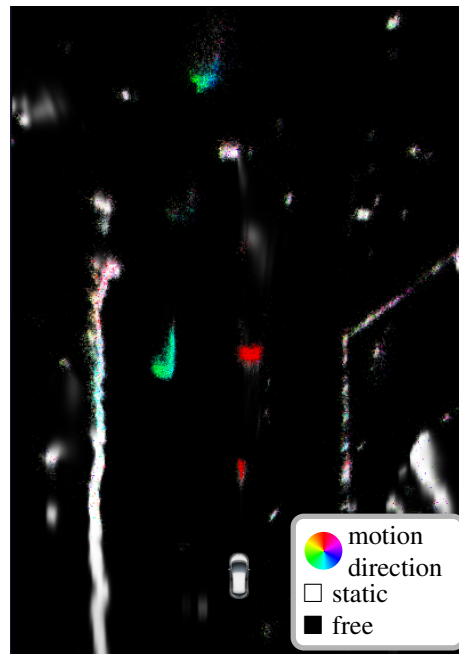
Figure 2 – Example of a Dynamic Occupancy Grid as provided by the CMCDOT perception suite [RPNL17, RNL15]. This image has been provided by [RDGML22].
