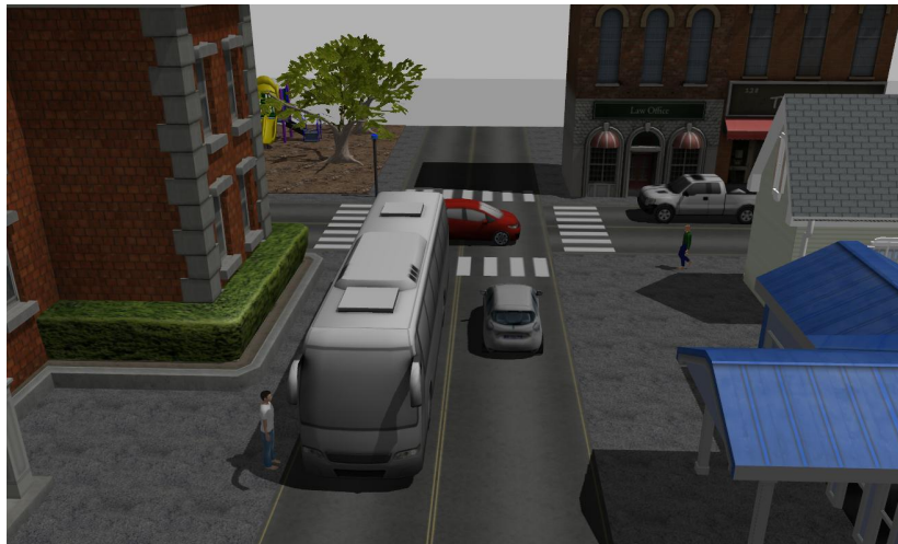
Figure 53 – Visualization of a simulated environment with the virtual twin of the experimental automated car (in gray, in the center of the image).
