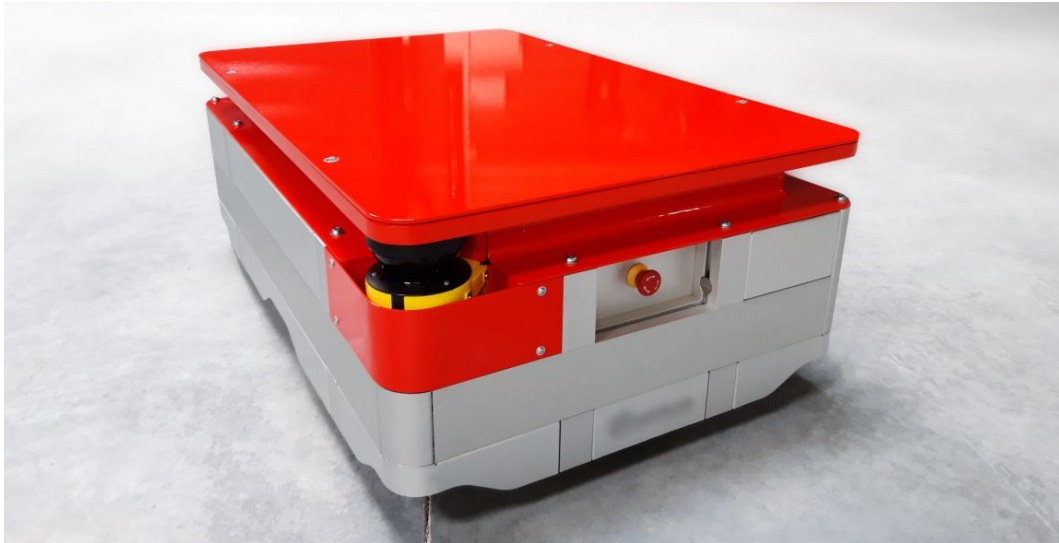
Figure 57 – The prototype of industrial indoor robot that has been used to experiment and demonstrate collision avoidance software contributions of this thesis. This robot is 90 cm long and 60 cm wide.
