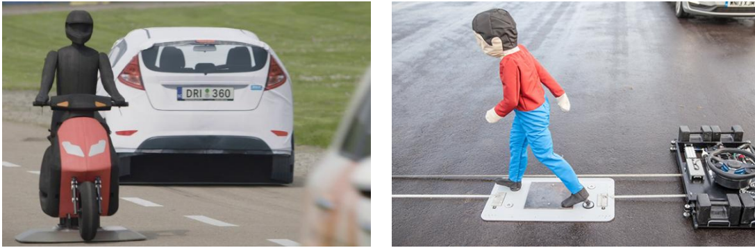
Figure 40 – These pictures display some examples of actuated dummies and soft targets that are used to test ADS and ADAS . These images are from www.abdynamics.com [A23].
