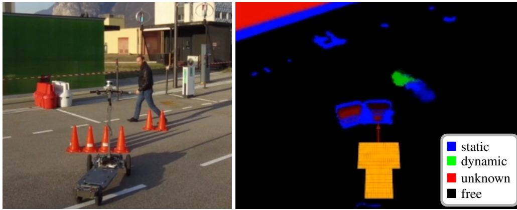
Figure 9 – Real world example of fused perception with the urban light vehicle prototype . The Dynamic Occupancy Grid gathers observations from different sensors and sensing modalities to accurately represent the scene.
