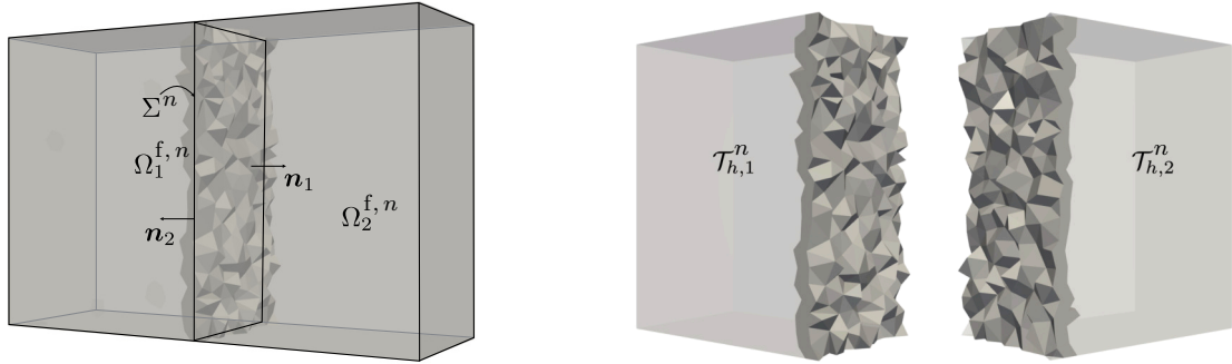
(a) Three-dimensional fluid and solid domains with the fluid intersected elements highlighted.
