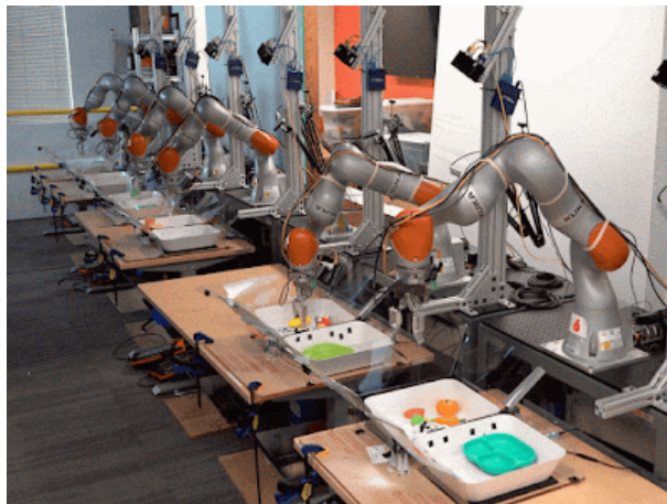
Figure 1.4 – Training reinforcement learning algorithms on real robots typically requires a large number of interactions, careful design of reward functions, and automatic reset mechanisms. Despite these efforts, the resulting policies are often confined to controlled lab environments.
