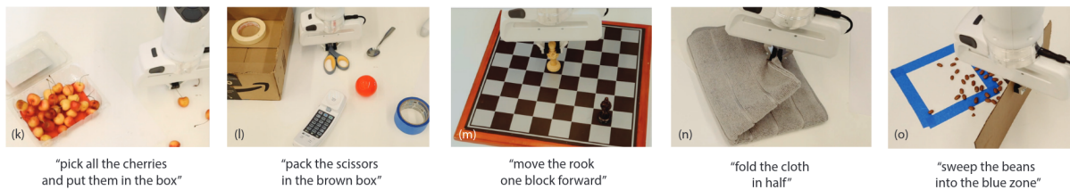
Figure 2.5 – CLIPort (Shridhar et al., 2022) uses pretrained CLIP (Radford et al., 2021) image and text encoders to perform language-conditioned visual manipulation tasks.
