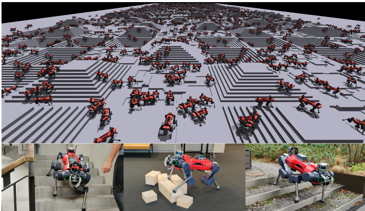
Figure 2.4 – Rudin et al. (2022) learns locomotion policies with reinforcement learning in massively paralleled simulations (top) that can transfer to real quadruped robots (bottom).
