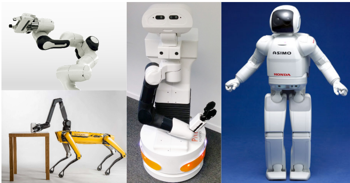
Figure 1.2 – Examples of available robot platforms that can physically perform various skills. From left to right: Franka Emika, Boston Dynamics’s Spot, PAL Robotics’ TIAGo and Honda’s Asimo
