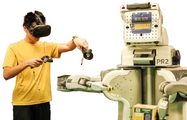
Figure 2.1 – Teleoperation is an effective way to collect data for robot learning (Zhang et al., 2018).
