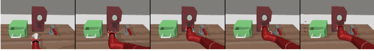
(a) Failure to close the drawer. Given a prompt of a human closing the drawer, the policy performs a pushing motion on the wrong object.
