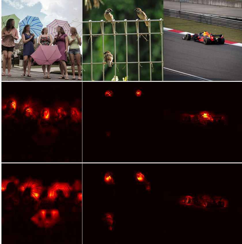
Figure 3.6 – Visualization of the attention map between the CLS token and individual patches in the class-attention stage. For each column, each row represents the attention map w.r.t. one head, corresponding to the image in the first row. Each head seems salient to semantically coherent regions. Heads are sensitive to similar features within the same or across images ( e.g. people or bird faces). They trigger on different concepts when such features are missing ( e.g. , cockpit for race cars).
