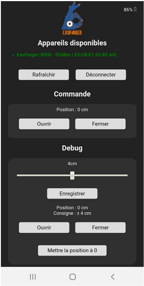
Figure 2.15: Android application to adjust and use Exofinger.
