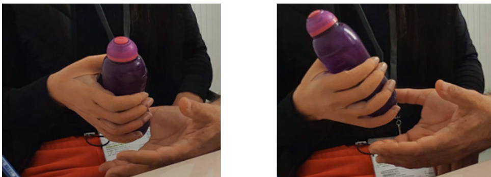
Figure 4.1: P7 of Exofinger holding the bottle for 7 seconds in neutral position (left) and more than 30 seconds using supination (right).
