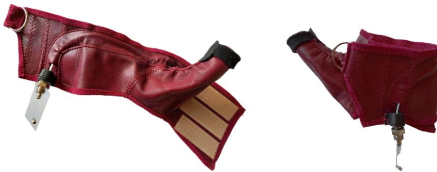
Figure 2.11: The Exofinger unfolded (left) is donned by wrapping (right) it around the hand.
