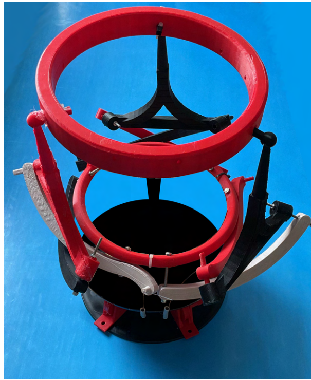
Figure 4.14: A rapid prototype for gauging the ROM and test actuation via cables.
