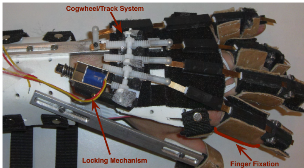
Figure 3.2: Prototype of a hybrid orthosis for assisting the power grasp from [118].
