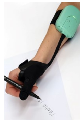
(d) Motorized thumb orthosis for key grip assistance. This device is expected to be available on the market at some point [108].
