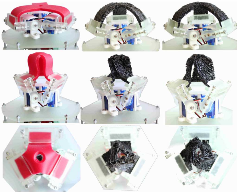
Figure 5.1: Three tripods with different mechanical properties. The middle and right components have anisotropy leading to a rotation when each segment of the tripod is brought together. source: [173]
