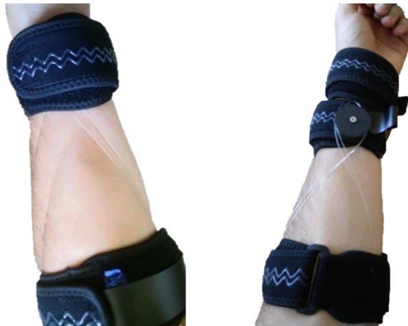
Figure 4.6: Test with wristbands and cables: winding cable around the forearm (left) and angle redirection utilizing a pulley (right).
