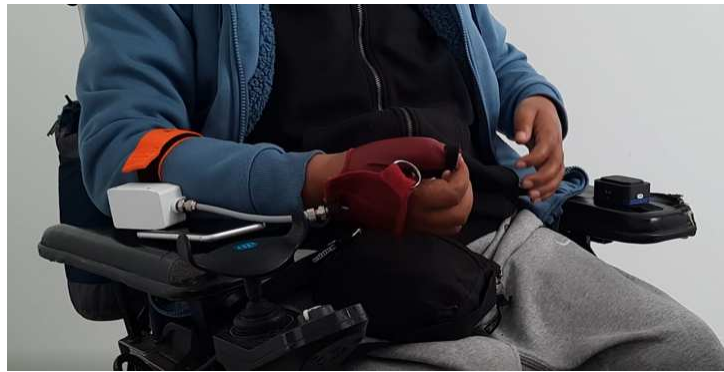
Figure 2.6: A participant wearing Exofinger on the right hand with the push button located on the opposite armrest.
