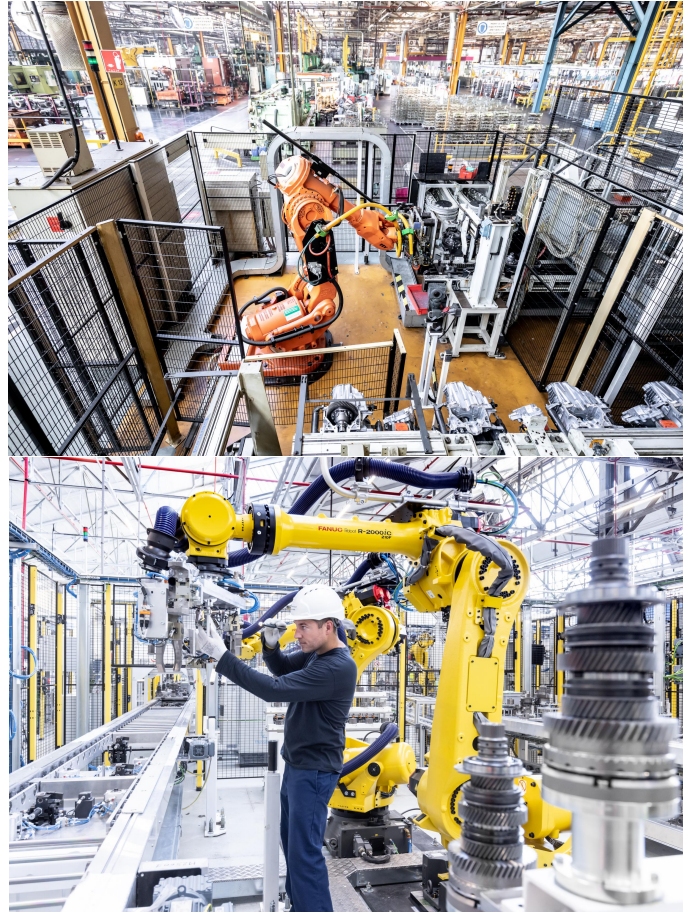
Figure 1.3: Example of a robot deployed inside a cage. Obtained from [Groupe PSA Communication Metz Tremery, 2018]; [Stellantis Communication, 2022a].
