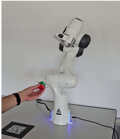
Figure 5.10: Showcases the interactive scenario (as defined in Section 5.4.3) used for the experiments, showing the robot tracking the pose of a plastic piece in real time. The video shows the experiment.
