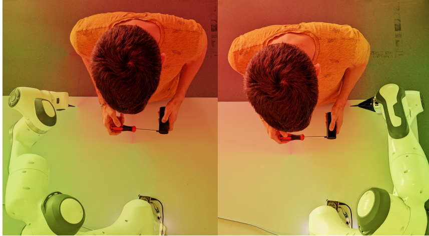
Figure 3.4: Safe workspaces in a collaborative environment cannot be defined with static zones as it depends on the robot-operator states and tasks.
