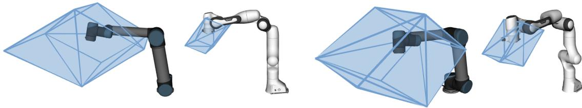
FIGURE 3.21: Two different views of Panda ( $n = 7$ ) and UR5 ( $n = 6$ ) robot's force polytope ( $m = 3$ ) calculated using the VEPOLI<sup>2</sup> algorithm. Both robots and polytopes are shown in the same scale (1m : 1000N). The figure shows that the UR5 has much larger polytope than Panda robot. This is due to its larger force capacity, as UR5 is rated for 5kg loads whereas Panda is rated for 3kg loads.
