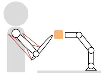
FIGURE 2.3: A collaborative example scenario where a human and a robot interact over an object fixed rigidly in the end-effector of the robot and in the hand of the human.
