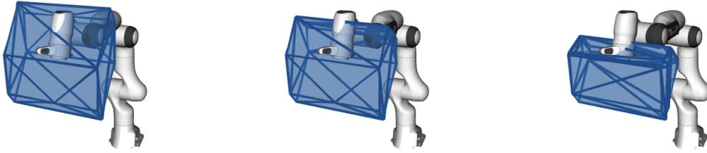
FIGURE 5.5: Reachable space polytope  $\mathcal{P}_x$  for a Franka Emika Panda robot for three different carried object masses (left to right)  $m_{object} = 0, 2$  and  $5\text{kg}$ , horizon time used  $t_h=0.15\text{s}$ .
