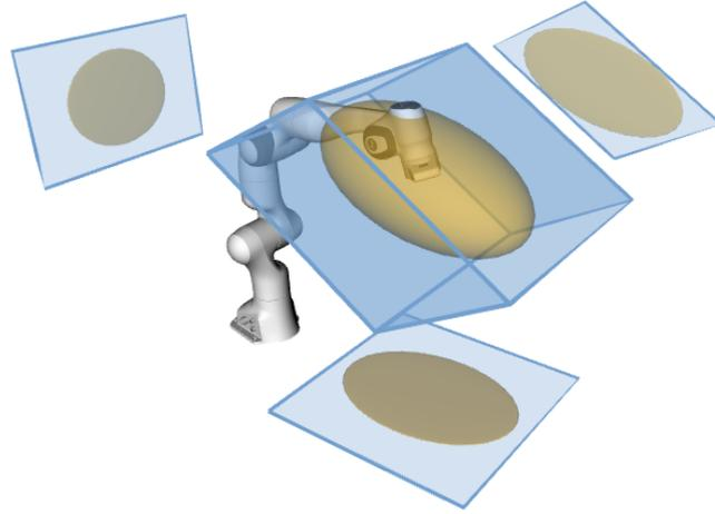
FIGURE 7.2: 2D and 3D force polytopes and their ellipsoid counterparts for a 7 degrees of freedom (DOF) Franka Emika Panda robot. Both polytopes and ellipsoids are calculated separately for the 3D and for each of the 2D reduced task-space cases. Both polytopes and ellipsoids take in consideration the true joint torque limits provided by the manufacturer. The underestimation of the true force capabilities of the robot by ellipsoids appears clearly.
