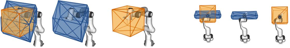
FIGURE 5.11: Comparison of the end-effector reachable space approximation using the convex polytope  $\mathcal{P}_x$  (blue) and the cube  $\mathcal{C}_x$  (orange) for the Panda robot with the horizon time  $t_h=200\text{ms}$ .
