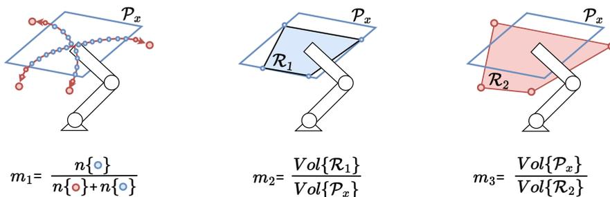
FIGURE 5.10: Depiction of the defined quantitative metrics for a simple 2 link planar robot. The notation  $n\{\cdot\}$  represents the number of points.
