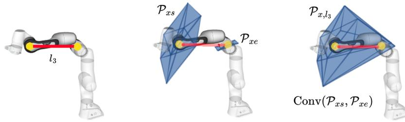
FIGURE 5.7: The figure shows the construction of the reachable space polytope of the Panda robot's link 3,  $\mathcal{P}_{x,l_3}$ . The first image shows the robot's link 3 modelled as a line segment  $l_3$  (in red). The polytopes  $\mathcal{P}_{x_s}$  and  $\mathcal{P}_{x_e}$  calculated in its vertices (yellow) are shown in the middle.  $\mathcal{P}_{x,l_3}$ , calculated as their Convex-Hull, is shown on the right. Robot is in its initial configuration, and the horizon time used is 150ms.
