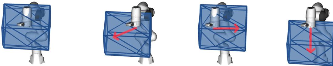
FIGURE 5.4: Reachable space polytope  $\mathcal{P}_x$  for a Franka Emika Panda robot's end-effector for 4 different end-effector velocities  $\dot{\mathbf{x}}_o = J\dot{\mathbf{q}}_o$  (from left to right)  $\dot{\mathbf{x}}_o = [0, 0, 0], [0, -1, -0.5], [0, 1, 0]$  and  $[0, 0, -1]m/s$ .
