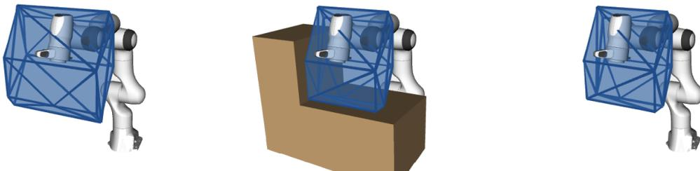
FIGURE 5.6: Resulting reachable space polytope  $\mathcal{P}_x$  for a Franka Emika Panda robot's end-effector when integrating the environmental constraints, horizon time used is  $t_h=0.15\text{s}$ . Environment is defined as  $z \geq 0.5\text{m}$  and  $y \geq -0.2\text{m}$ .
