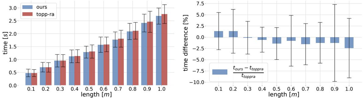
FIGURE 6.15: Plots showing the comparison of the trajectory execution time of the proposed method with TOPP-RA, for trajectory lengths ranging from  $d = 0.1$  to  $1m$ . Left graph shows the comparison of the execution time, while the graph on the right shows the difference in execution time in a form of percentage. Means and variances are calculated over 100 random trajectories.
