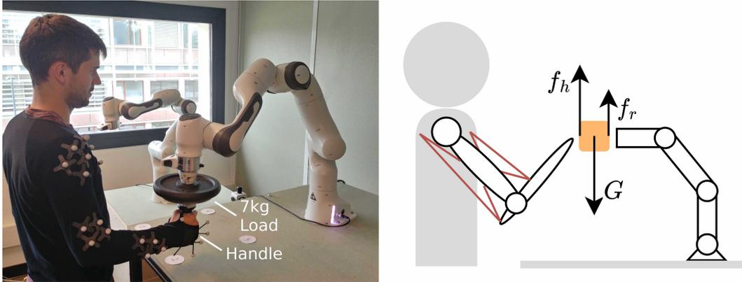
FIGURE 4.7: This figure show the experimental setup. The robot end-effector is fixed to the carried object and the human operator is holding the object by the handle. The object's mass is  $m = 7\text{kg}$ , while the operator and the robot collaborate to compensate the full weight of the object.
