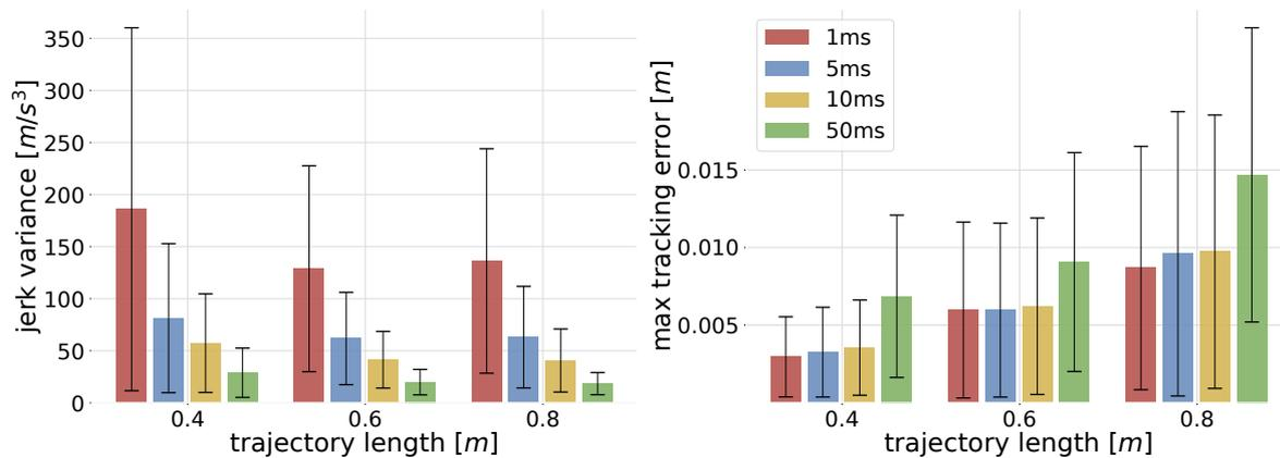
FIGURE 6.12: Plots showing the comparison of the jerk variance (left) and tracking error (right) of the proposed method with and without oscillation compensation, for trajectory lengths  $d = 0.4, 0.6$  and  $0.8m$ . Means and variances are calculated over 100 random trajectories. Four down-sampling times are compared  $\Delta t_p = 1, 5, 10$  and  $50ms$ .
