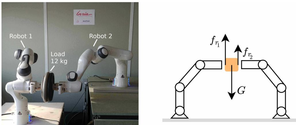
FIGURE 4.2: Figure showing the experimental setup for dual robot arm collaborative carrying. Two Franka Emika Panda robots jointly carry the object with a mass of  $m = 12\text{kg}$ , where each object compensates for a part of the total weight  $\mathbf{f}_{r_1} + \mathbf{f}_{r_2} = m\mathbf{g}$ . The object is rigidly fixed in the end-effectors of both robots.
