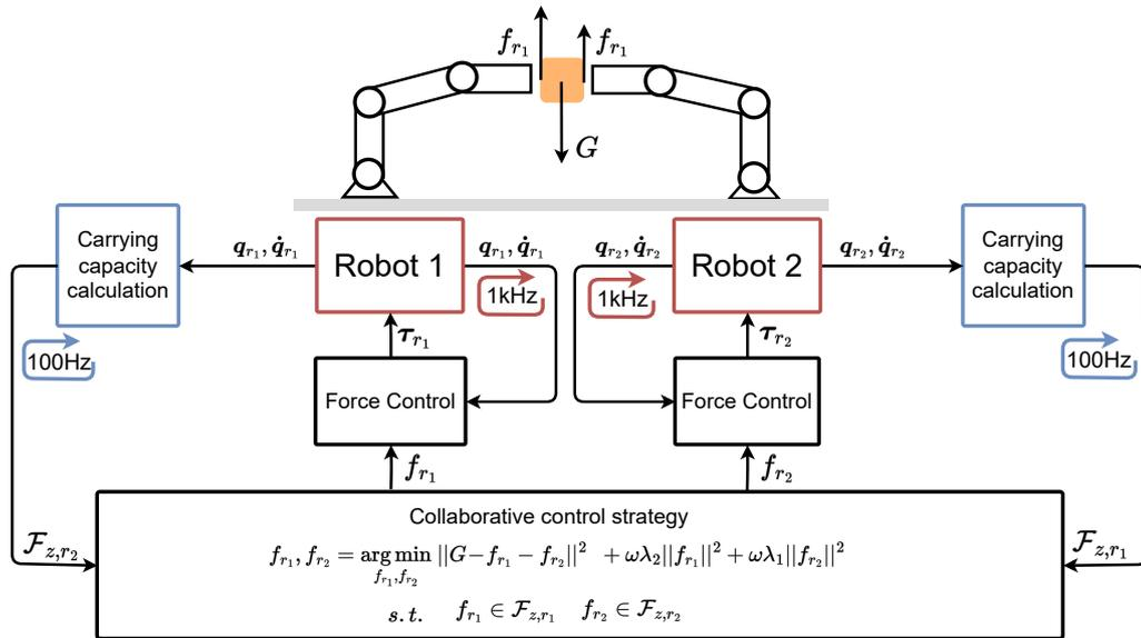
FIGURE 4.4: The block diagram showing the implemented robot control scheme. Each robot's low-level force control loop runs at 1kHz, while the carrying capacity calculation and the collaborative control strategy are evaluated at the frequency of 100Hz.
