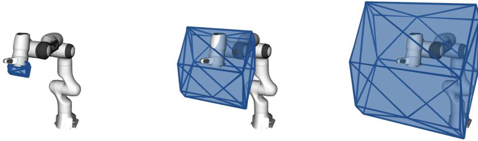
FIGURE 5.2: Three images show the comparison of the size of the reachable space polytope  $\mathcal{P}_x$  of a Franka Emika Panda<sup>3</sup> robot's end-effector for 3 horizons (left to right)  $t_h = 0.05, 0.15$  and  $0.25s$ , for the same configuration.
