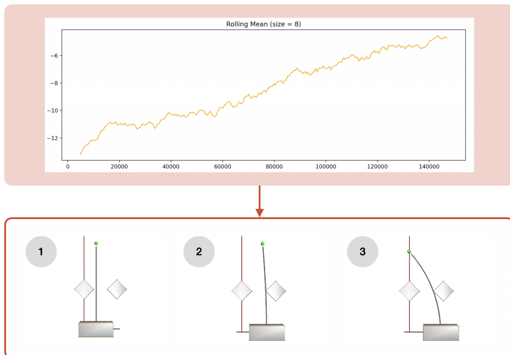
Fig. 3.12: Solving the CartStemContact problem using the SAC algorithm. Top: cumulative reward. Bottom: solving steps. 1) Random goal and base positions. 2) Using the opposite contact to deform the beam. 3) Solving the positioning task.
