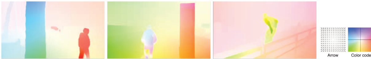
Figure 1.1 – Examples of parallax motion in natural scenes. Optical flow fields colored with the HSV color code [59] are shown on the bottom right. From left to right: two flows from our outdoor videos, one flow from a parkour sequence in Davis. In the left sequence, the parallax motion is the apparent motion of the tree trunk, in the center sequence the apparent motion of the pole, and in the right sequence, it is the motion of the fence.
