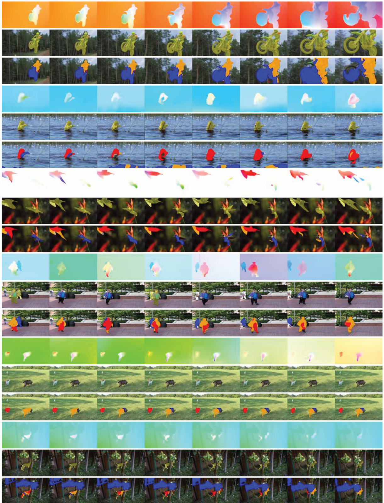
Figure 4.7 – Results obtained with our LT-MS-K4 method, i.e., using four masks ( K = 4 ). Six groups of results are displayed. For each group, we have three rows. The first row samples successive flow fields corresponding to the processed video, the optical flow fields being represented using the usual HSV color code. The second row contains the corresponding images of the video, where the ground-truth segment corresponding to the moving object is overlaid in yellow when available at that frame. The third row shows the motion segments provided by our LT-MS-K4 method (given by layers that are not necessarily connected) with one colour per segment. For all the results, we adopt the same color set for the three masks corresponding to the moving objects (blue, red and orange), and we let the background image for the background mask for the sake of clarity. These examples are drawn from the different datasets.
