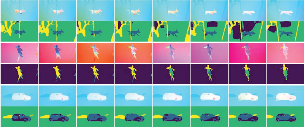
Figure 2.6 – Illustration of the implicit temporal consistency ensured (to some extent) by our method with four masks. For each group, first row: input optical flow fields displayed with the HSV color code, second row: OFS maps. The color code is the same for all segmentation maps (dark blue: mask 1, light blue: mask 2, green: mask 3, yellow: mask 4). Examples are drawn from DAVIS2016 (from top to bottom): libby , dance-twirl , and car-roundabout videos.
