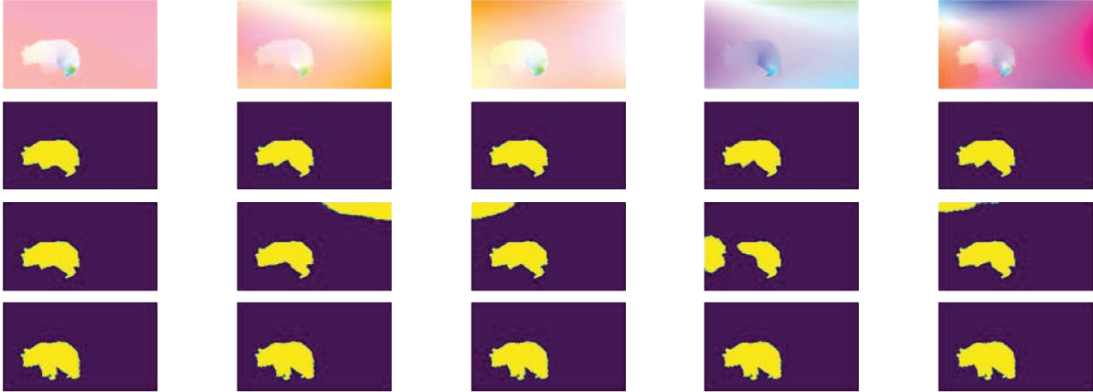
Figure 7.1 – Data augmentation adding a quadratic global motion on the optical flow field. From top to bottom : Optical flow field displayed with the usual HSV code [59]; Predicted mask with our network trained using data augmentation; Predicted mask with our network trained without data augmentation; Ground-truth segmentation mask.
