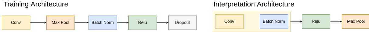
Figure 5.1 – Modification of the ordering of the network inner layers. Left: Order for training and test. Right: Order for interpretation. Weights of each layer remain unchanged. For interpretation, Convolution and Batch Norm layers are merged into a functionally equivalent convolutional layer.
