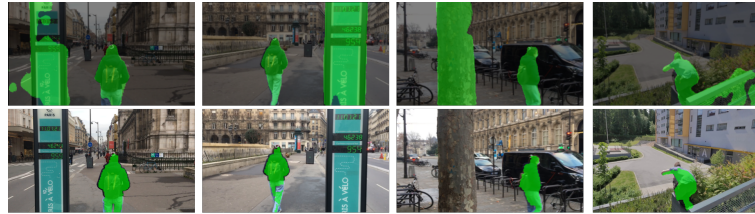
Figure 5.3 – Extracted salient masks, superimposed on original images, on three examples from our dataset and one from DAVIS2016 ( parkour video). Top row : results from [47] using the available code and model (without the postprocessing step). Bottom row : corresponding results using our method (NIMS). CIS [47] detects the foreground static object due to parallax motion, while our method successfully discards it.
