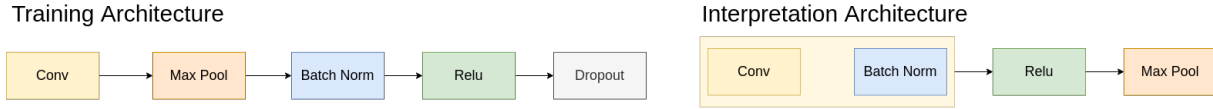
Figure 5.1 – Modification of the ordering of the network inner layers. Left: Order for training and test. Right: Order for interpretation. Weights of each layer remain unchanged. For interpretation, Convolution and Batch Norm layers are merged into a functionally equivalent convolutional layer.
