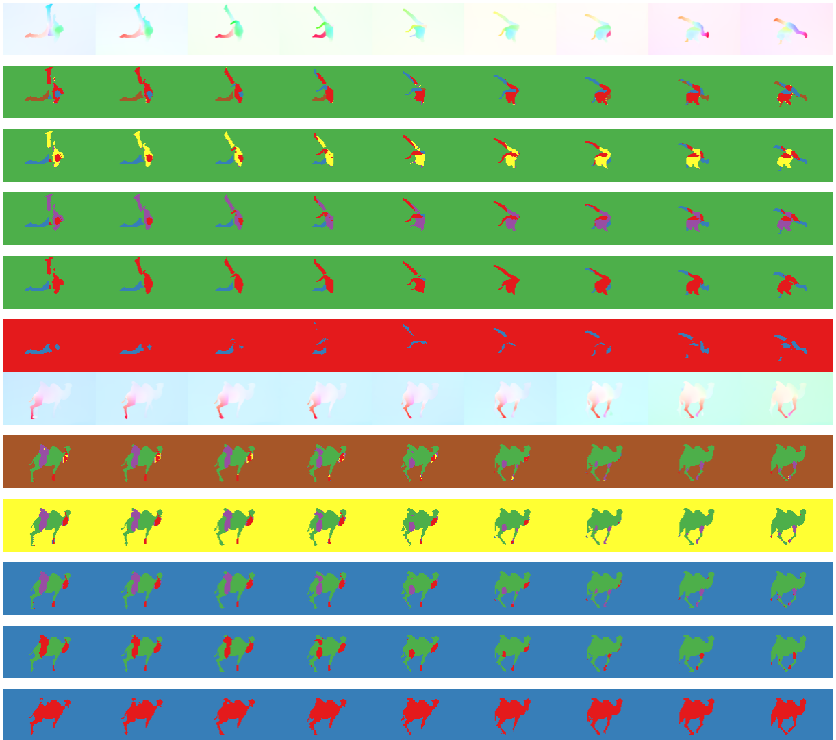
Figure 7.8 – Qualitative results obtained with LT-MS-SA (including the slot attention decoder) with a variable number of masks at inference time. The first row of the two groups of results is the optical flow field (HSV color code), then, from top to bottom, we display the motion segmentation from 6 to 2 masks using the same model. In order to push the model to keep coherent labels across levels, we keep the same set of initial queries and give only the requested number for each level as input. The two sequences are breakdance-flare and camel from the DAVIS2016 dataset.
