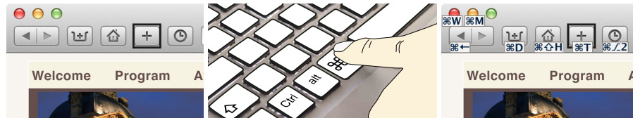
Figure 3.2: The user wants to open a new tab but is not sure of the hotkey. He visually locates the button in the toolbar (boxed on left), then presses the Command key (Cmd) to activate ExposeHK, which overlays toolbar items with available keyboard shortcuts (right). He completes the command by pressing Cmd+T.
