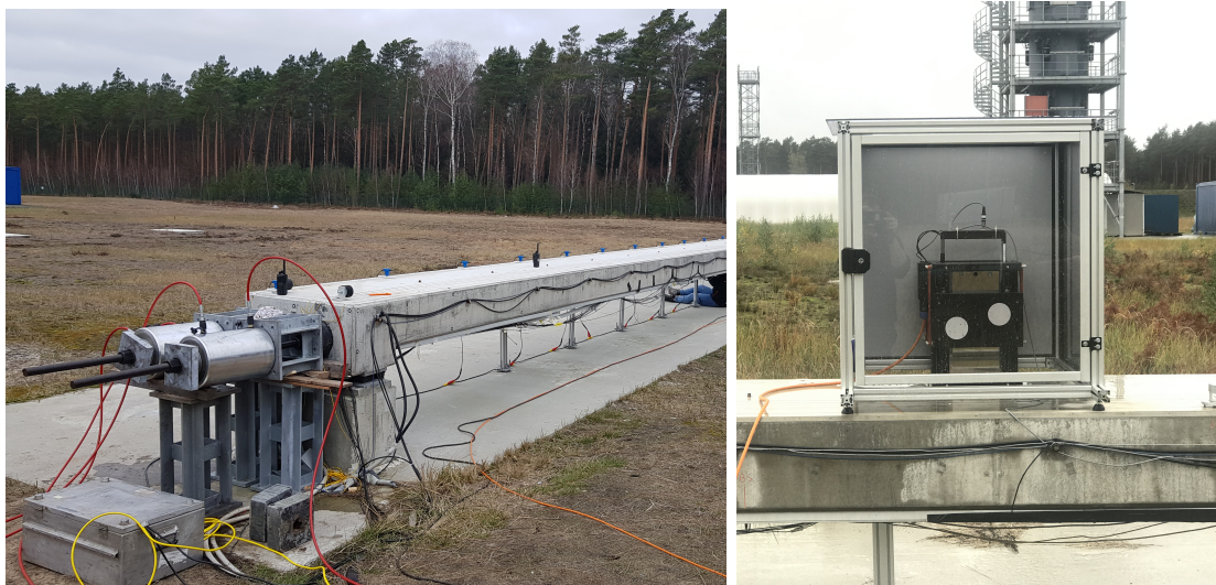
Figure 7.3 – Pre-stressing facility (left) and encased shaker (right).
