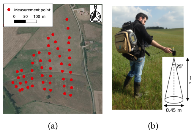
Figure 1.4.: (a) Example of S-shaped pattern within the grassland. The red dots correspond to the sampling plots. The plots are at least 10 meters from the boundaries. The plot positions were acquired with a GPS device with a precision of around 2-3 meters. The background is an aerial photograph from the French orthophoto database "BD Ortho" ©IGN. (b) Schematic of the measure acquired with a sensor with a field-of-view of 25^\circ at a height of one meter above ground.
