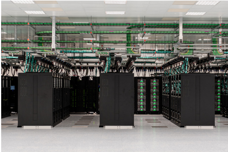
Figure 1.3: HPC facility at ECMWF, made up of four Atos BullSequana XH2000 clusters 2
