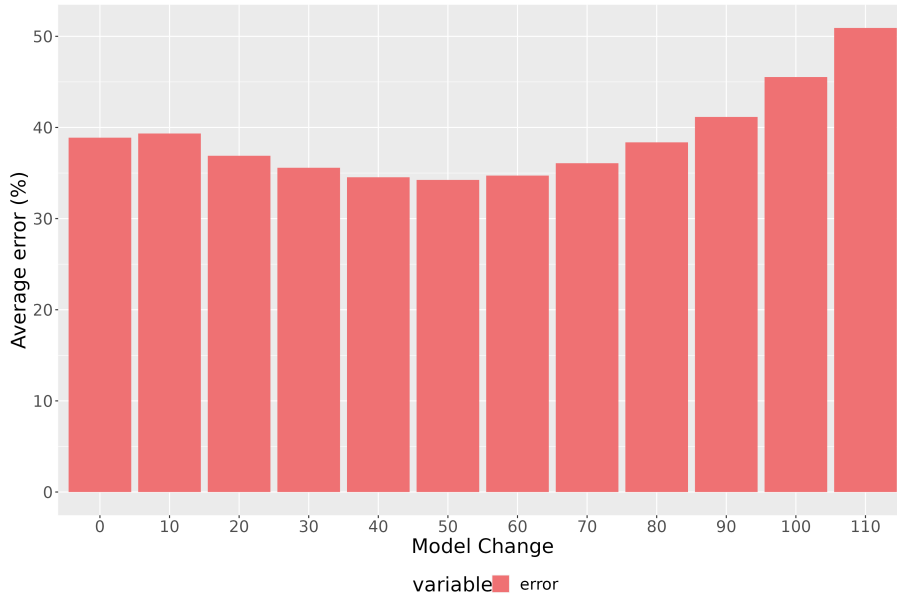
Figure 6.13: Average error across synchronous OSU benchmarks, as a function of when we switch our network model (32 processes)
