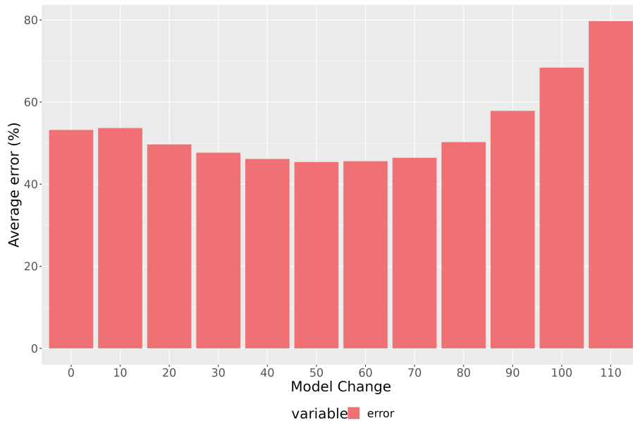
Figure 6.15: Average error across asynchronous OSU benchmarks, as a function of when we switch our network model (32 processes)
