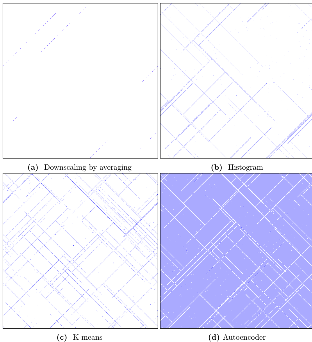
Figure 5.8 – Qualitative comparison of coarse-graining methods Simulations are on grids of 4096 \times 4096 cells coarse-grained to 512 \times 512 . Most lines are barely visible with downscaling 5.8a, but are visible in 5.8b-5.8d. Coarse-graining helps visualize linear structures that would be hard to see otherwise.
