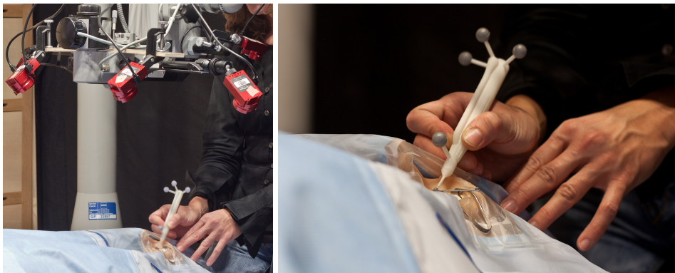
Fig. 1.16: Overview of our setup: mannequin and microscope where 6 infrared cameras are attached. These cameras allow to track in real-time the motion of the surgical tools.
