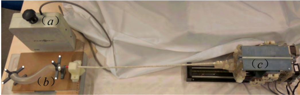
Fig. 3.15: Experimental setup for the motion control of a catheter robot through contacts. (a) NDI electromagnetic tracking system: Aurora; (b) a rigid tube for the experiment. The white points are the feature points which are used for the calibration; (c) the cable-driven continuum catheter robot which has four step motors to actuate the bending and one step motor to control the insertion.
