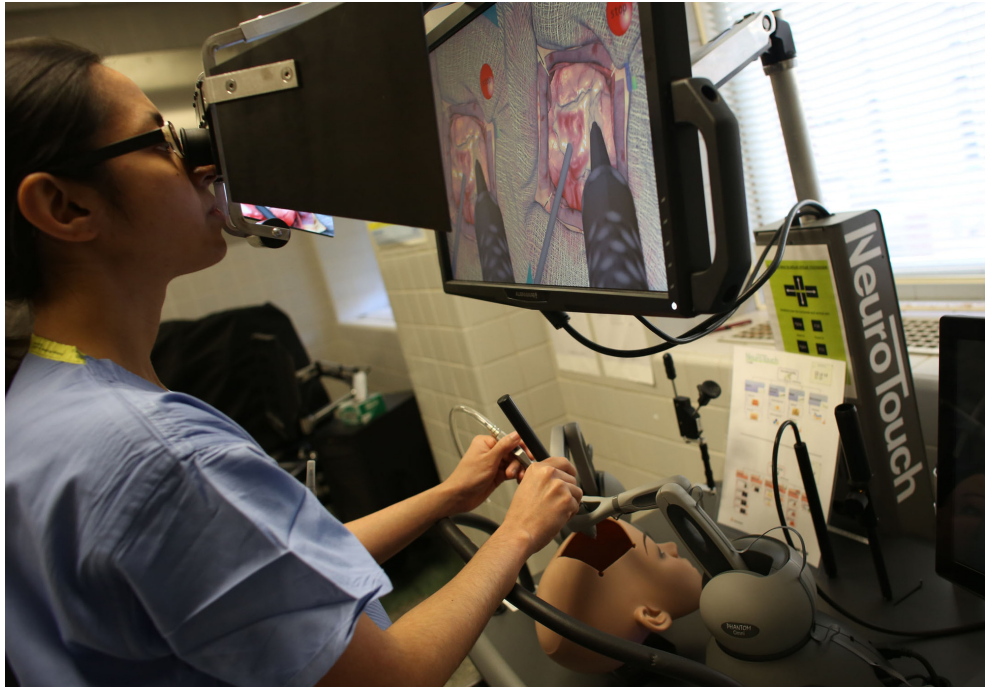
Fig. 1.3: Example of a neuro-surgical training system by Neurotouch©. The system includes robotic arm equipped with stylus (Geomagic© Touch) to acquire user gesture and to render forces in case of contact and a stereo-vision display to mimic the use of binoculars.
