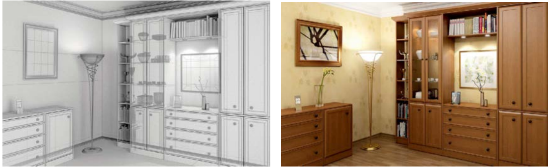
Figure 1.2: Traditional rendering uses artist-generated scene assets such as a triangular mesh (left) for geometry, and complex material and illumination models to render the scene using a path tracer (right).
