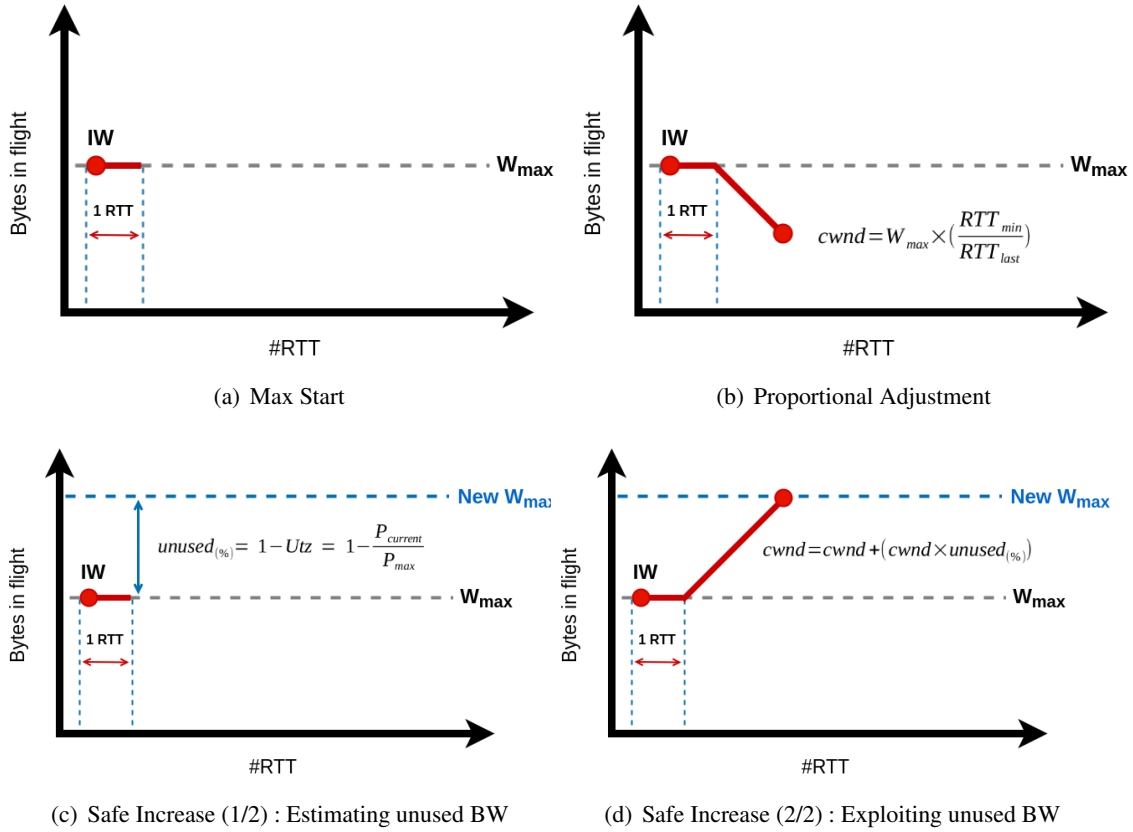
Figure 3.5 – Congestion Window evolution during the three operating states of SIGMA
