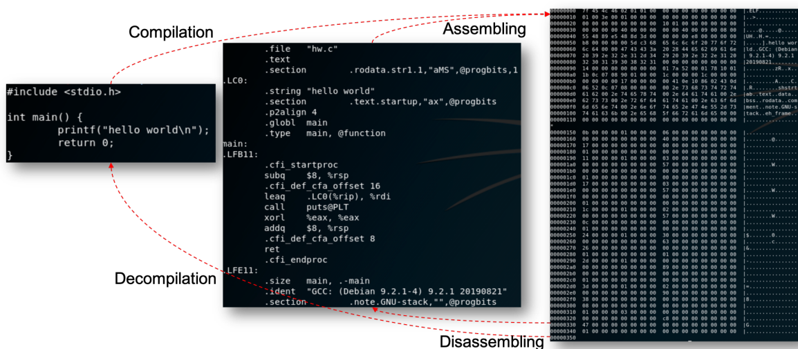
Figure 2.17 – [De]compilation and [de]assembling of a “hello word” code in C.
