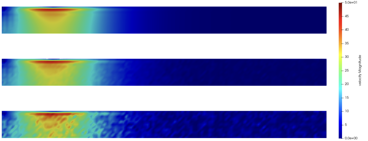
Figure 3.4: The data at t_{50} . From top to bottom: ground truth without noise, \delta_{\text{noise}} = 1\% , and \delta_{\text{noise}} = 15\%
