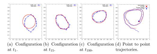
Figure 2.22: Vesicle configuration (blue) at  $t_n$ , n = 1, 69, 199 against the solution (red). Right hand side : trajectory of a point in the estimation (blue) compared to the one of the presumed tracked point in the real vesicle (red) at final iteration. Parameters :  $\kappa = 10$ ,  $\kappa_{obs}\delta = 0.1, \sigma = 6.0, \sigma_v = 0.075$
