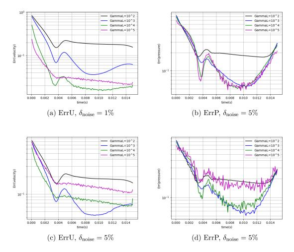
Figure 3.16: Relative error for the velocity and the pressure estimations, for  $\gamma_M = 10^3$  with noisy data,  $\delta_{\text{noise}}$  parametrizes the percentage of noise.
