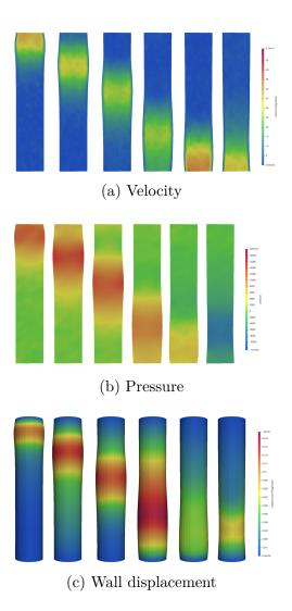
Figure 4.21: FSI state estimation using Algorithm 6 with (Eulerian) noisy data (5%) at  $t_{30}, t_{50}, t_{70}, t_{100}, t_{120}$  and  $t_{140}$ .
