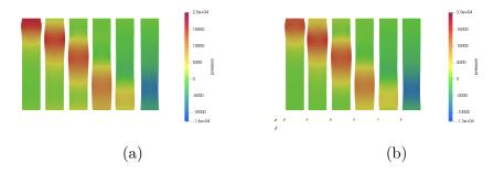
Figure 4.15: Snapshots of the pressure estimation for the two types of boundary conditions,  $\gamma_{\rm M} = 10^4$ ,  $\gamma_{\rm f} = 10^4$ , (Eulerian velocity data). (a) Inflow Dirichlet/Outflow Neumann. (b) Inflow Neumann/Outflow Neumann.
