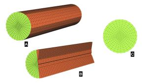
Figure 4.2: Reference geometric configuration. (A) View of the 3D cylinder, colored by surface label ( $\hat{\Gamma}_{in}$  in green,  $\hat{\Sigma}$  in red. (B) Plane cut visualization with tetrahedra (y = 0). (C) Mesh of the circular basis.
