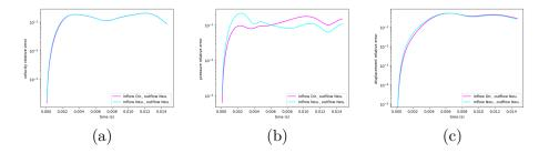
Figure 4.16: Comparison of the relative errors for two types of boundary conditions,  $\gamma_{\rm M} = 10^4$ ,  $\gamma_{\rm f} = 10^4$  (Eulerian velocity data). (a) Velocity. (b) Pressure. (c) Fluid domain displacement.
