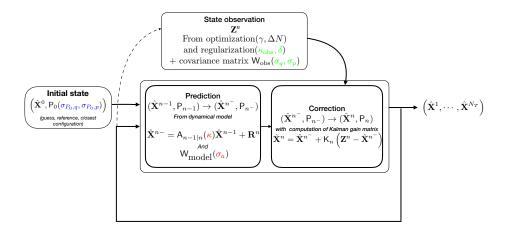
Figure 2.5: The parameters of the Kalman filter and the state observation.
