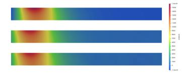
Figure 3.11: Estimated pressure at  $t_{50}$ .  $\gamma_M = 10^3$ , for 1% noise (middle), 5% noise (bottom). The reference solution is given on top.
