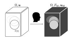
Figure 2.2: The surface  $\Gamma(t)$  is transported by  $\boldsymbol{u}$  within the domain  $\Omega$ .  $\Gamma(t)$  is sufficiently detectable on the image sequences  $F_{\rm M}$  and  $\boldsymbol{u}_{\rm M}$  is a measurement of the velocity field  $\boldsymbol{u}$ .
