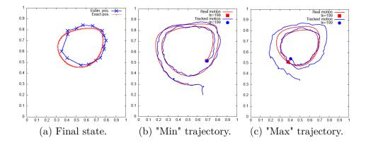
Figure 2.15: Simulation for  $\sigma = 2.0$ ,  $\sigma_v = 0.105$ ,  $\sigma_q = 1.5$ . Red : real vesicle. Blue : estimation by the method.  $\kappa = 10$ ,  $\kappa_{\rm obs}\delta = 0.1$ .
