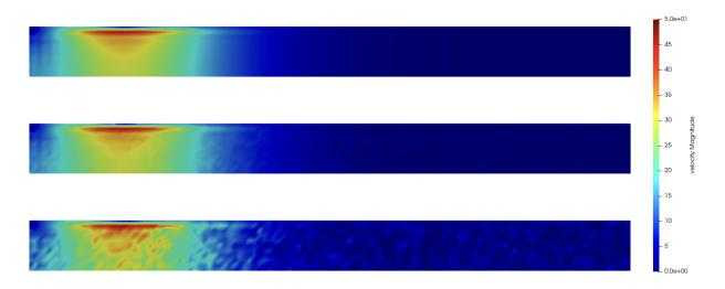
Figure 3.4: The data at  $t_{50}$ . From top to bottom: ground truth without noise,  $\delta_{\text{noise}} = 1\%$ , and  $\delta_{\text{noise}} = 15\%$
