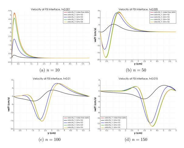
Figure 3.12: Vertical velocity at the interface, with noise-free data
