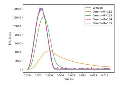
Figure 3.9: Estimated inflow pressure profiles with 1% noise in the measurements
