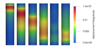
Figure 4.5: Snapshots of the wall displacement (reference solution) at  $t_{30}$ ,  $t_{50}$ ,  $t_{70}$ ,  $t_{100}$ ,  $t_{120}$  and  $t_{140}$ .
