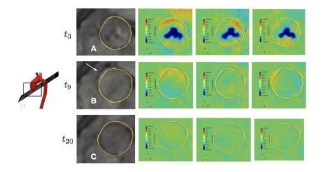
Figure 2.31: Slice cut view, at the inlet of the geometry. On the left, the position of the plane for slice visualization. On the right, the slice cut at 3 time iterations : A)  $t_3$ , B) $t_9$  is the end of the systolic phase, C)  $t_{20}$  during the diastolic phase. The best Dice reconstruction is in green, one of the 3 average Dice reconstruction in yellow, and the worst Dice case is in red.
