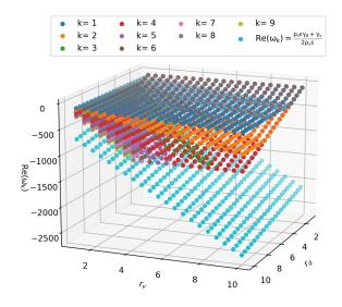
Figure 4.27:  $\max_{n=1,2} \{ \operatorname{Re}(\omega_{k,n}) \}$ , for  $\gamma_{f} = 100, R = 0.5, L = 5$ .
