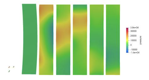
Figure 4.33: Estimated pressure with Algorithm 8 for  $\gamma_M = 10^5$ ,  $\gamma_f = 50$ ,  $\gamma_{sdf} = 2000$  and  $\gamma_{dvf} = 200$ , at  $t_0$ ,  $t_{30}$ ,  $t_{50}$ ,  $t_{70}$ ,  $t_{100}$ ,  $t_{120}$  and  $t_{140}$ . The displacement has not been amplified
