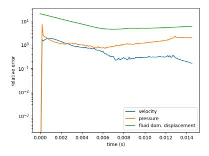
Figure 4.34: Relative error in the velocity, the pressure and the (fluid domain) displacement for  $\gamma_M = 10^5$ ,  $\gamma_{\rm f} = 50$ ,  $\gamma_{\rm sdf} = 2000$  and  $\gamma_{\rm dvf} = 200$ .
