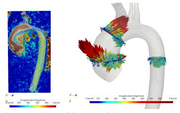
(a) Slice view of the ve-(b) velocity field visualization at 3 locity magnitude. slice cuts.
