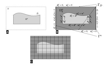
Figure 4.8: 2D sketch of the Eulerian velocity data generation. (A) Reference domains in dashed lines. (B) Extension to  $\Omega_2^n := \mathcal{V} \setminus \Omega^n$ . (C) Interpolation on the hexahedral grid.
