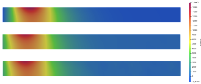
Figure 3.11: Estimated pressure at t_{50} . \gamma_M = 10^3 , for 1% noise (middle), 5% noise (bottom). The reference solution is given on top.
