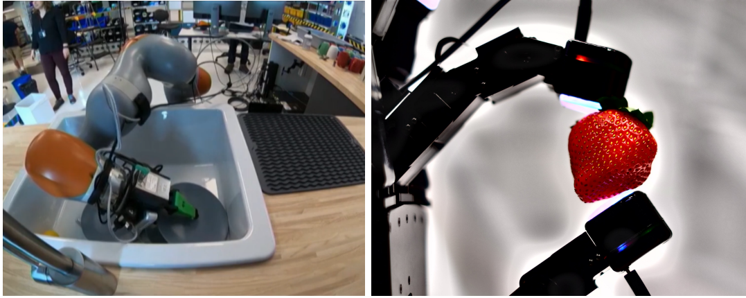
Figure 1.3: Precise manipulation tasks involving sensing and contact. These tasks are challenging because they require millimeter-precise controller with close-loop sensor feedback, a particularly daunting problem as we lack general approaches to design or learn such controllers.
