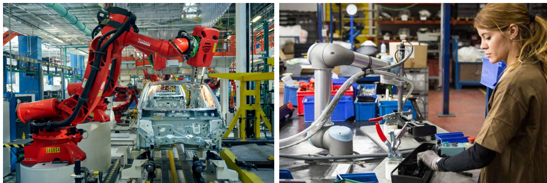
Figure 1.2: (Left) Robots performing specific tasks, such as welding pieces of a car, in a constrained environment. Industrial robots are highly specialised and are designed to perform one or a few fixed tasks. Each task requires the development of a new controller by highly skilled engineers. (Right) A collaborative robot, helping a person crafting an object. To get there, we need general controllers using vision to solve a rich variety of tasks and react with changes in the environment.
