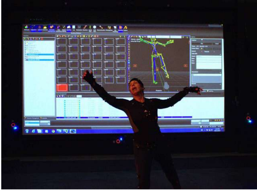
Figure 3.4. The data collection using EMGs, an accelerometer, and a Vicon Motion Capture
