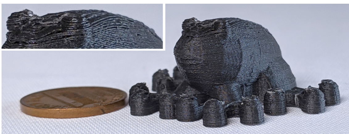
Figure 74: Small frog model printed with curved slicing on an Anet A8 printer, with a 0.4mm nozzle and 103 layers between 0.3mm and 0.05mm. Layers at the top smoothly follow the curvature.
