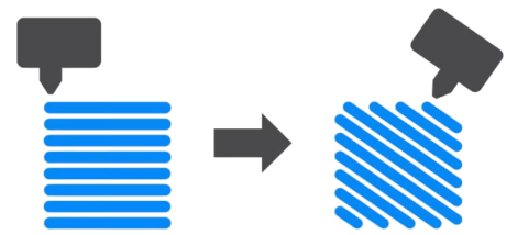
(b) Left: Standard FDM extrusion Right: Belt 3D tilted extrusion
