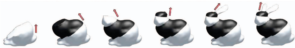
Figure 41: Different parts of the Stanford bunny model are fabricated in different directions (following the red arrows in the illustration), and filaments of different colors are used for making different parts by the RoboFDM system [Wu, Dai, Fang, Liu and Wang, 2017].
