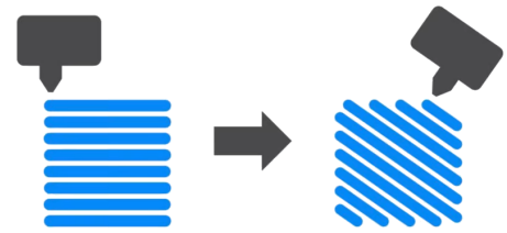
(b) Left: Standard FDM extrusion Right: Belt 3D tilted extrusion
