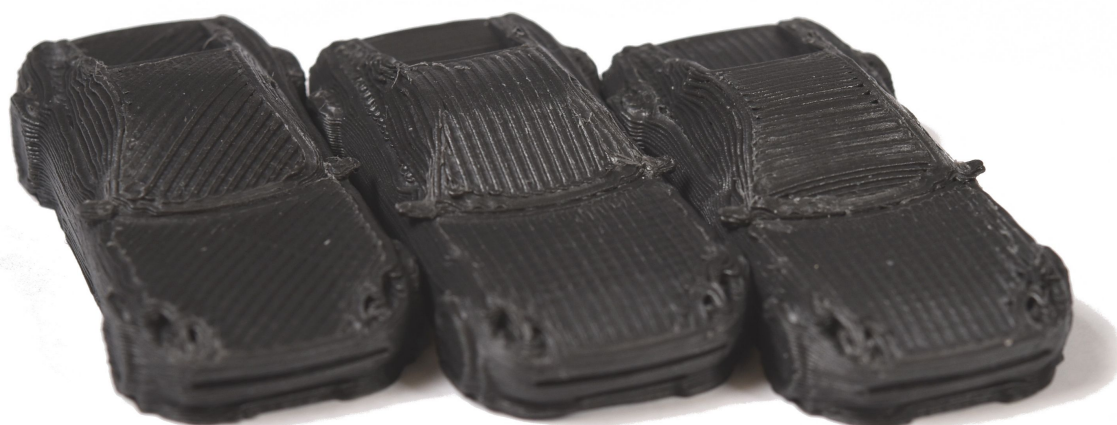
Figure 81: Different toolpath orientations for the top layers in curved slicing result in different surface finish. The visible stripes are shallower than the layer thickness, yet they create a visual effect that is detrimental to perceived quality. The effect also depends on lighting and view angle.
