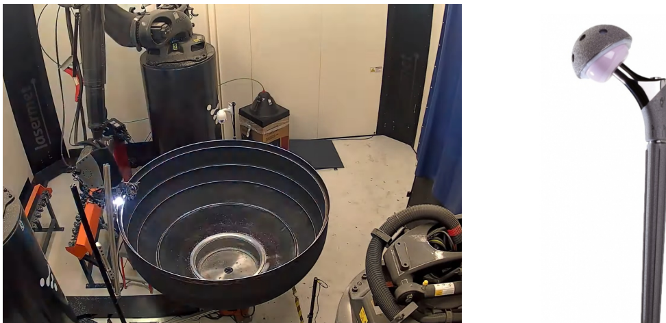
Figure 2: Example of technical prints. Left: Rocket tank being printed with a robotic arm. Right: A 3D-printed hip implant with a porous trabecular structure, which allows for the patient's bone tissue to integrate with the part. © Limacorporate
