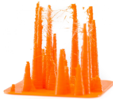
Figure 24: Stringing defect during travels.
