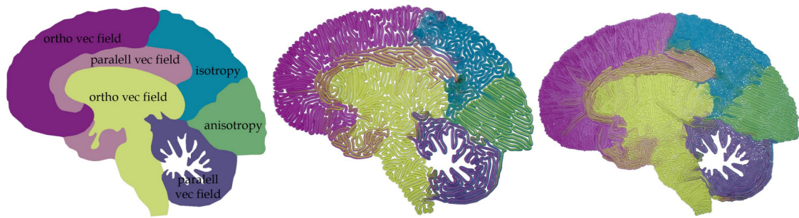
Figure 29: Dense Hamiltonian cycle infill with direction bias, isotropy, anisotropy, vector field alignment, and zoning [Bedel et al., 2022].
